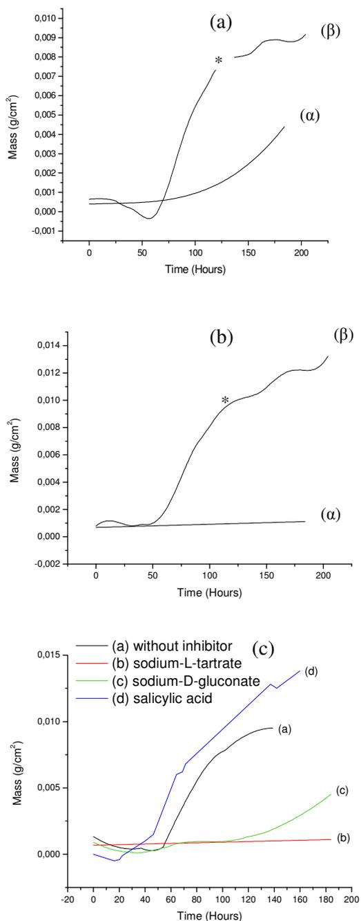
Fig. 4 Scale growth tests in synthetic Bayer liquor with addition of potential inhibitors: (a) Sodium-D-gluconate (1 mmol/L), (b) Sodium-L-tartrate (5 mmol/L), (c) comparison of all inhibitors; where inhibitors were added ( $\alpha$ ) before plunging the plate into the solution, ( $\beta$ ) after the crystal growth had begun (\*)
