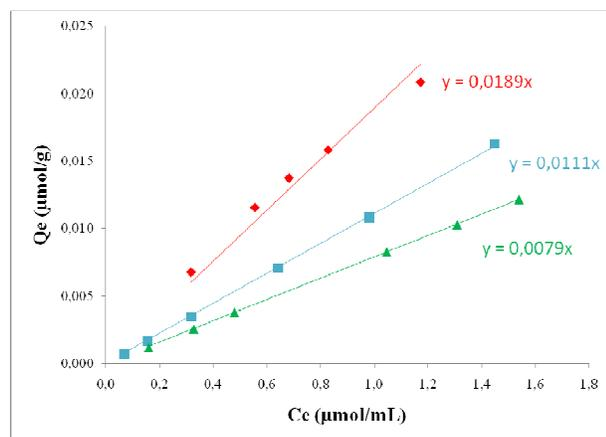
Fig. 3 Effect of molecules structure on adsorption on iron with NaOH 3M for (-▲-) Salicylic acid, (-■-) Sodium-D-gluconate, (-◆-) Sodium-L-tartrate.
