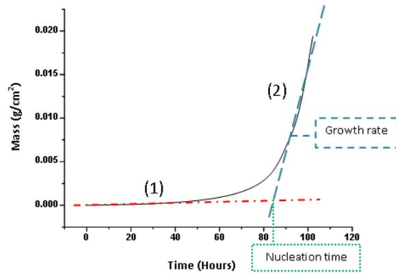
Fig. 2 Scale growth typical curve. (1) Scale nucleation, (2) Scale growth
