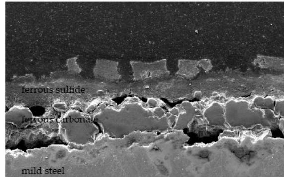
**Fig. 3 Cross Section of a corroded surface**
