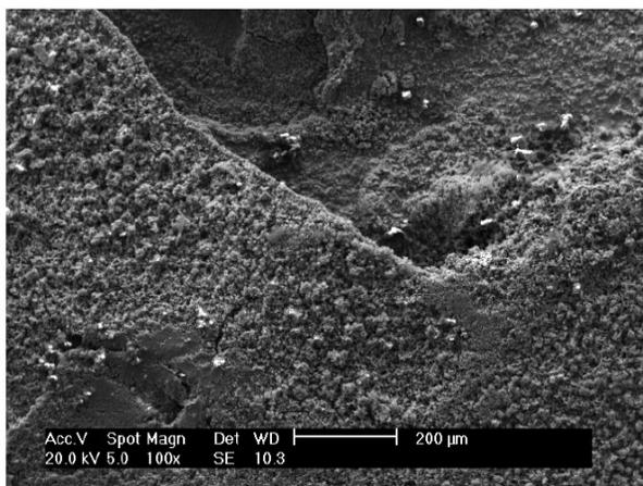
**Fig. 2 Top view of a corroded surface**
