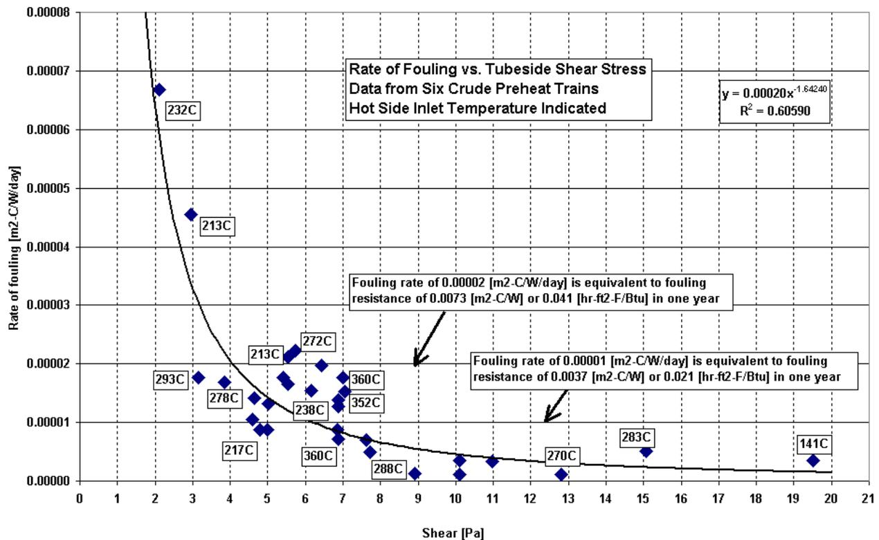
Fig. 1 Rate of Tubeside Fouling vs. Shear Stress and Velocity
