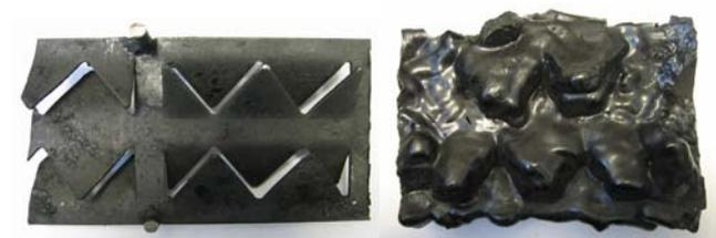
Figure 8 Segment of grid blade under clean and severely fouled conditions.
