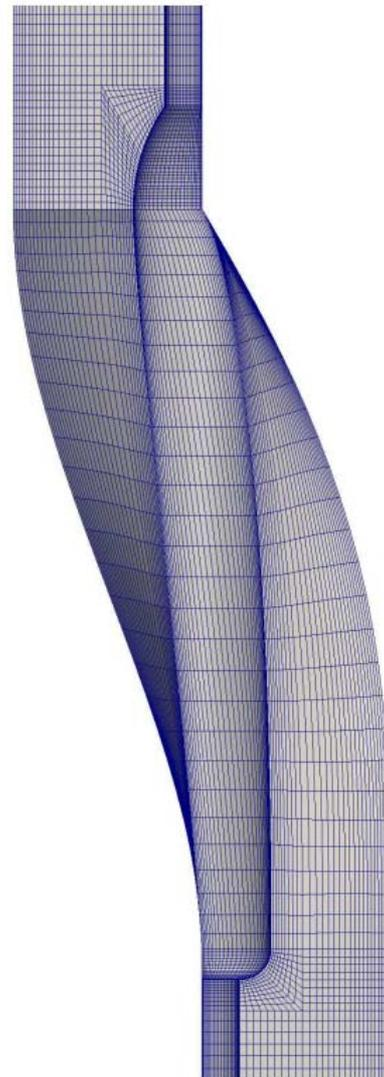
Fig. 4 An example mesh of the pipe, close to the swirling device
