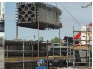
Figure 5. CC 106A being removed after 6 hours in the vessel
