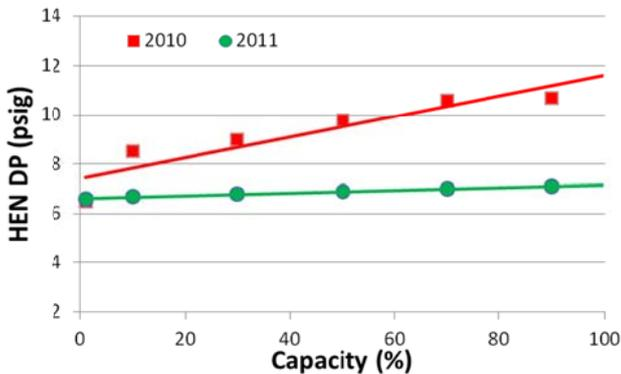
Figure 8. Differential Pressure (DP) vs. Flow Capacity (%) for the 8 unit Compabloc exchanger network, April 2010 vs Today<sup>i</sup>
