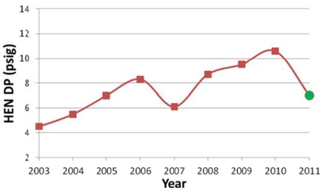
Figure 9. Compabloc (8 unit) exchanger network DP at 70% Capacity by Year (the last point is post cleaning of one exchanger and partial cleaning of three others during this study)<sup>i</sup>
