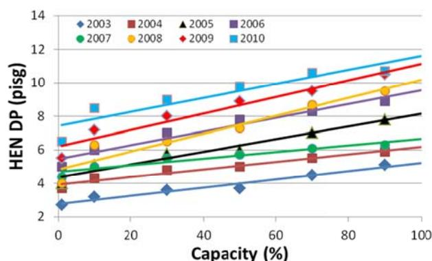
Figure 1. Differential Pressure (DP) vs. Flow Capacity (%) for the 8 unit Compabloc exchanger network by year
