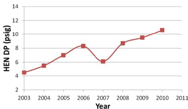
Figure 2. Compabloc exchanger network DP at 70% Capacity by Year
