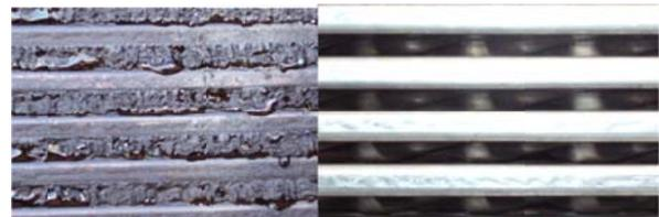
Figure 10. CC 106 D Compabloc exchanger before (a) and after (b) cleaning
