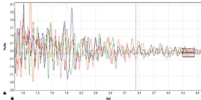
Fig. 3 Several signals taken from heavily fouled tubes
