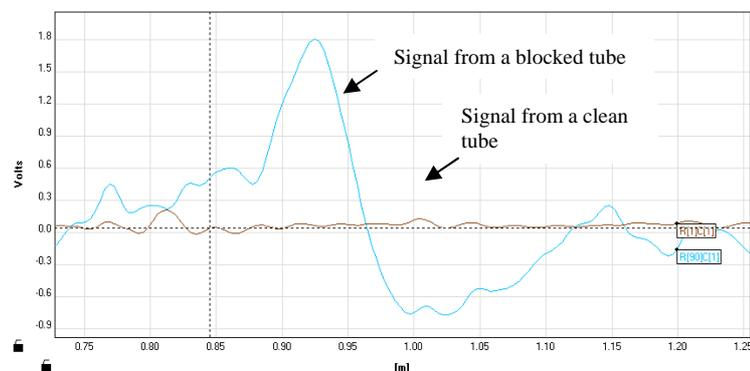
Fig. 2 Signals taken from a clean tube and a blocked tube
