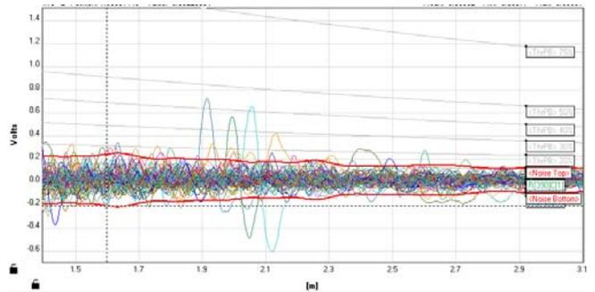
Fig. 9. 71 superimposed signals after cleaning with 10 ksi. Noise band is narrower with few isolated peaks.
