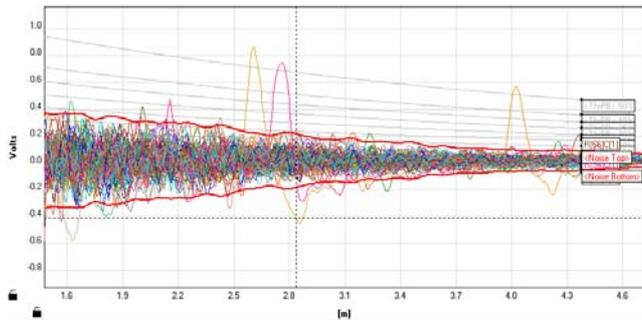
Fig. 5 Superimposed signals from 94 heavily fouled tubes, along with the resultant noise band, and the calculated blockage thresholds.
