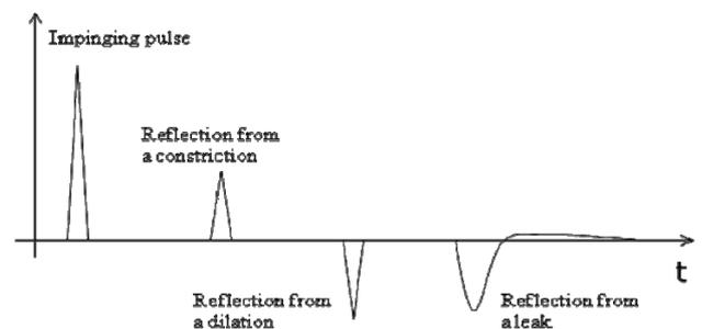
Fig. 1 Schematic examples of reflections from discontinuities
