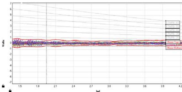
Fig. 6. Superimposed signals from 33 clean tubes, along with the resultant noise band, and the calculated blockage thresholds. The noise band is very narrow in this case.
