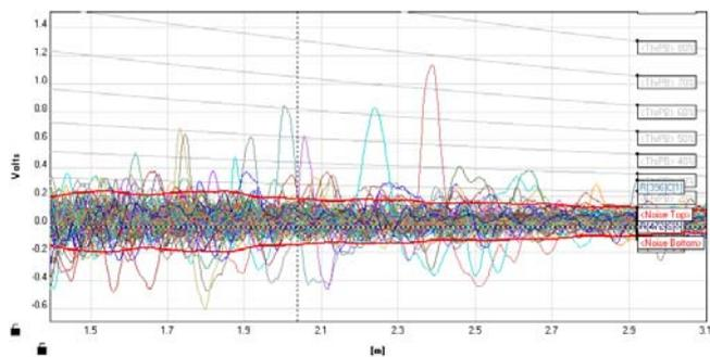
Fig. 7. 115 superimposed signals after partial cleaning, i.e. no main phase. Note the many isolated peaks.
