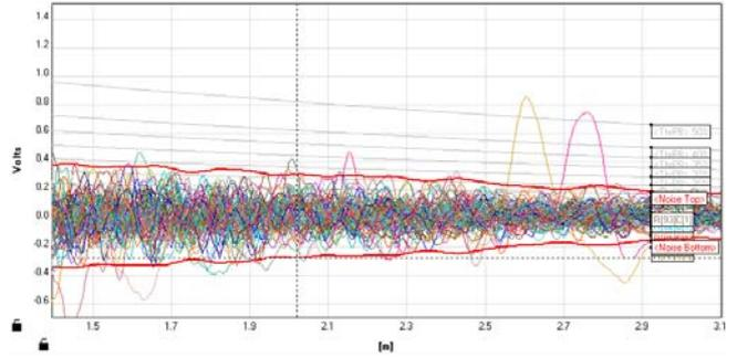
Fig 8. 94 superimposed signals after "standard" cleaning. Noise band is still wide, but fewer isolated peaks are present.
