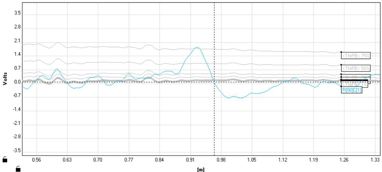
Figure 4 - A signal with a single blockage, along with thresholds (light grey) for determining blockage size
