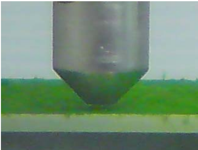
Figure 6 Gauging of a Synechococcus biofilm grown on perspex. Nozzle tube external diameter 6 mm.
