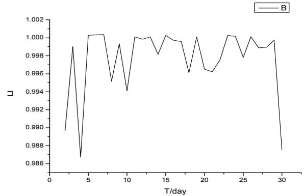
Fig.7 The value of LI when stainless steel immersed in the culture medium which contained SRB
