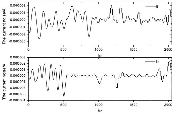
Fig.3 a.The current noise after stainless steel had been immersed in sterile medium for one day
