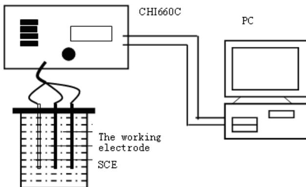
Fig.1 The experimental system
