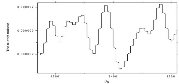
Fig.5 Enlarged picture of the current noise after stainless steel had been immersed in the culture medium which contained SRB for seven days
