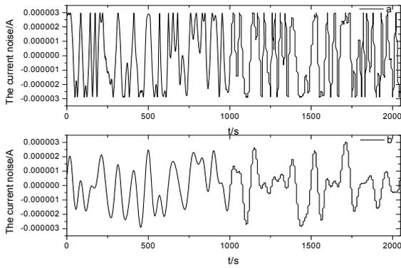
Fig.2 a.The original signal of current noise after stainless steel had been immersed in sterile medium for seven days
