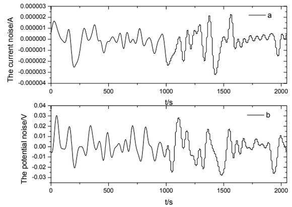
Fig.4 a.The current noise after stainless steel had been immersed in the culture medium which contained SRB for seven days
