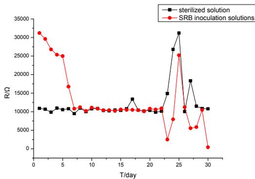
Fig.8 Noise resistance when stainless steel immersed in the culture medium which contained SRB
