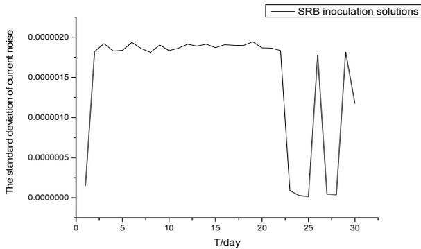
Fig.6 The standard deviation of current noise ( $S_I$ ) when stainless steel immersed in the culture medium which contained SRB
