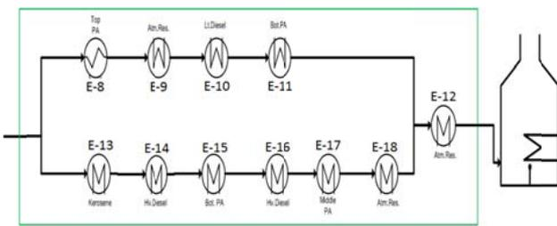
Figure 2: Second Preheat Train (downstream of desalter)
