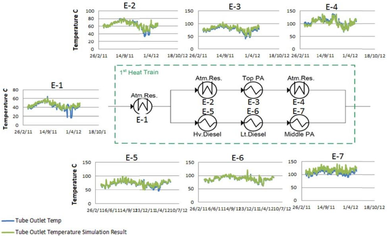
Figure 4: Operational and Simulated Tube Outlet Temperatures
