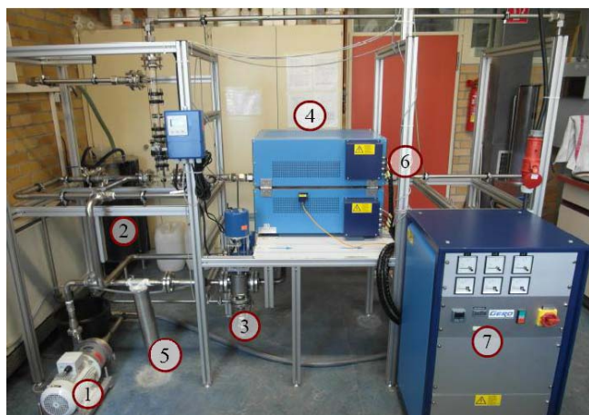
Fig. 2. A photo of the experimental setup; (1) 3 hp centrifugal pump, (2) 60 l water tank, (3) a 3 WV that is fully actuated by a motor and a flow controller, (4) a 10 kW electrical furnace, (5) 70 \mu\text{m} filter, (6) piping (7) control panel for the furnace.
