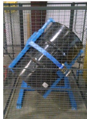
Fig. 5 Drum tumbler acquired by HTRI to mix crude oils
