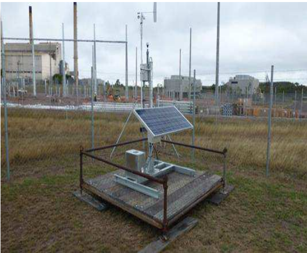
Fig. 1 The E-Sampler used for collecting the real time dust, weather conditions and dust samples
