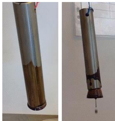
Figure 1: Following extraction from the crude oil:water test media, the liquids drain immediately from the coated tubes (right). The liquids remain on an uncoated tube section.
