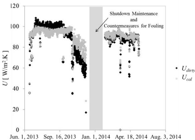
Figure 2 Comparison between  $U_{dirty}$  and  $U_{clean}$  profiles
