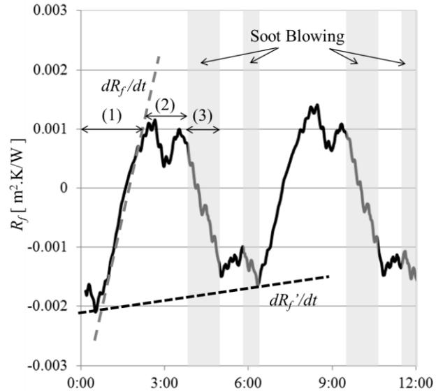
Figure 4 Profile of fouling resistance (2013/6/30)
