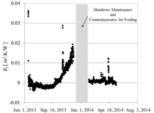
Figure 3 Profiles of fouling resistance
