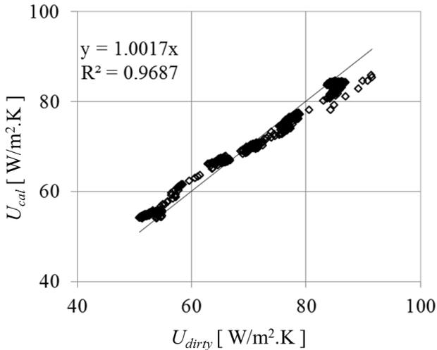
Figure 1 Comparison between  $U_{dirty}$  and  $U_{clean}$  during the exchanger's clean period
