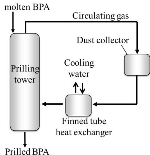
Fig. 1 process flow of prilling section
