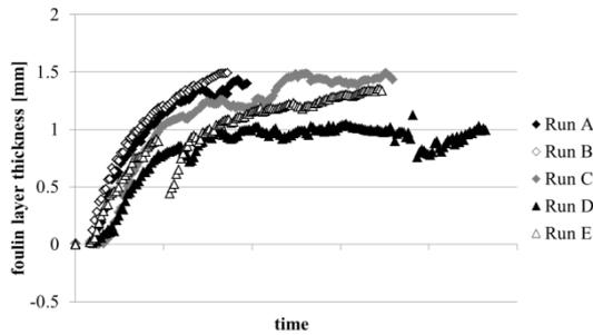
Fig. 6 Profiles of estimated fouling layer thickness
