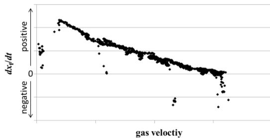
Fig. 10 Correlation between fouling rate and gas velocity calculated with current fouling thickness and flow rate
