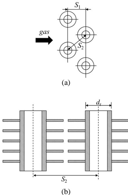
Fig. 3 Tube layout showing the parameters which affect the pressure drop
