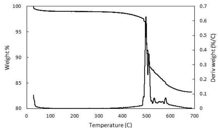
Fig. 1 TGA curve of HTSG coating measured in air.
