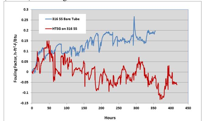
Fig. 4 Comparison of fouling rate for bare SS316 tube (blue) and tube coated with HTSG (red) at 600 °F in flowing crude oil
