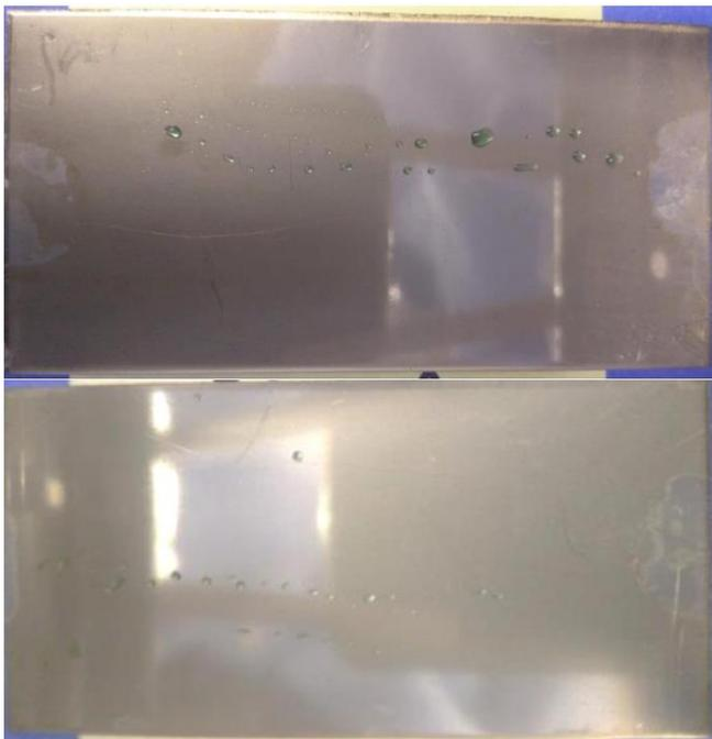
Fig. 3 Samples of HTSG coating after 6 h steam exposure
