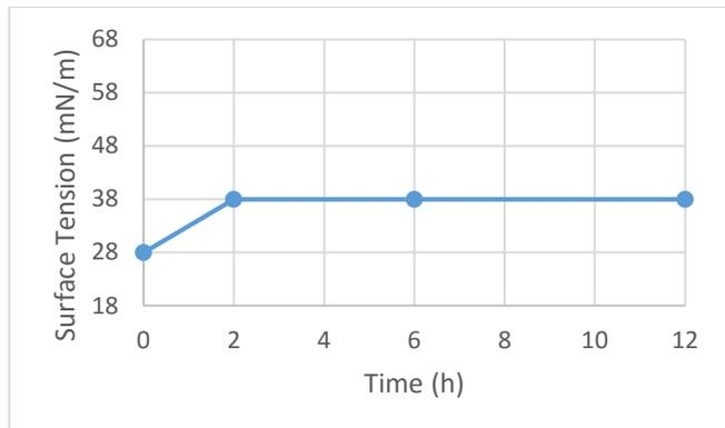
Fig. 2 Surface energy developments of the HTSG coating during steam out test (185 °C, 150 psig pressure).
