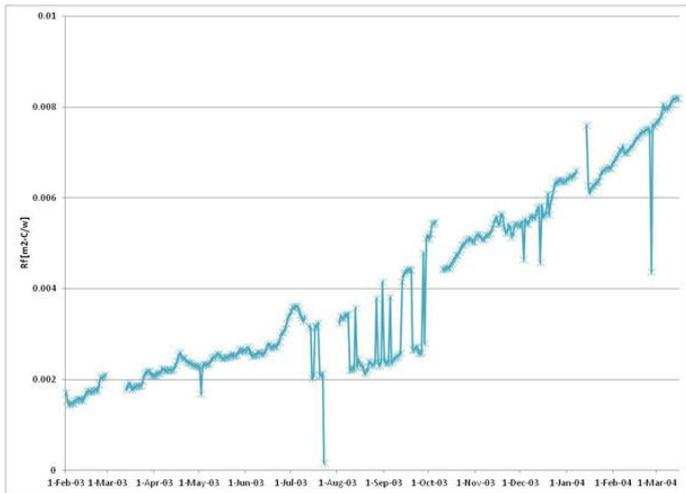
**Fig. 4 Fouling Resistance vs Time for an Operating Heat Exchanger – Example of Measurable Fouling Rate**
