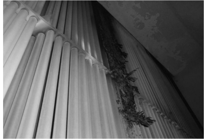
Fig. 5 Fouled shell side of the preheater; the black matter is, in fact, solidified PWG leaking into the shell-side through cracked U-tubes.
