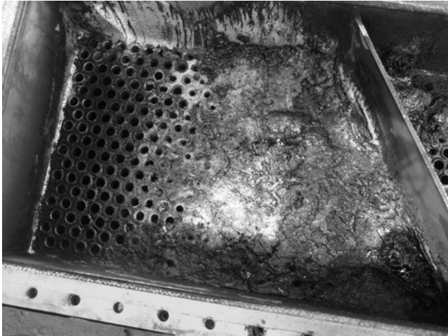
Fig. 3 Fouled inlet tube sheet
