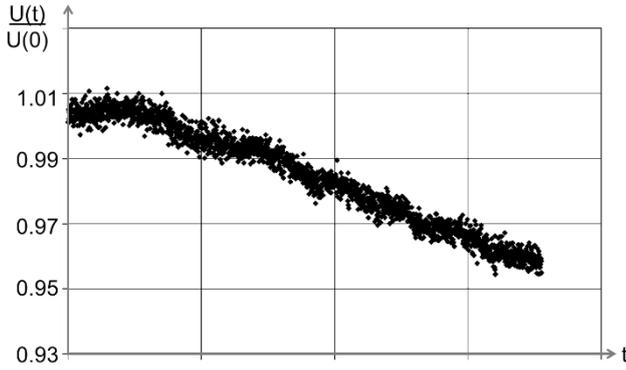
Fig. 3 Typical evolution of the overall heat transfer coefficient observed on the rig during a fouling test.
