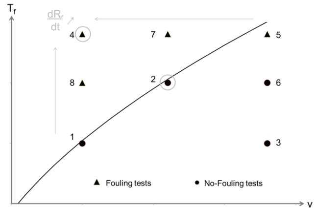
Fig. 2 Experimental plan and qualitative test results on the shell-and-tube heat exchanger (Crude A); circled tests were carried out with the two crudes.
