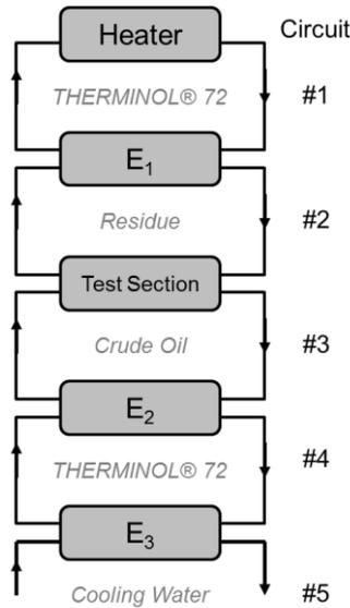
Fig. 1 Process flow diagram of the test rig.
