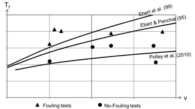
Fig. 4 Comparison of experimental results with fouling models; theoretically, the fouling points must be above the curve and no-fouling points, under or near the curve.
