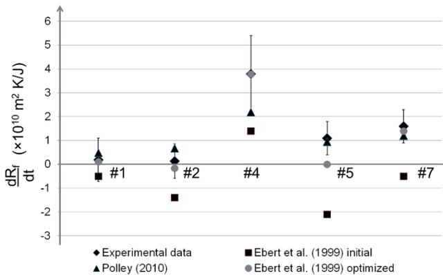
Fig. 7 Comparison of fouling rates predicted by the Ebert et al. (1999) and Polley (2010) models with experimental values.
