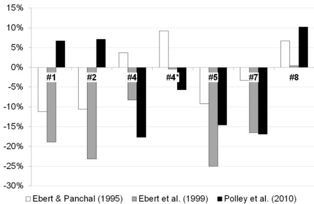
Fig. 5 Comparison between model predictions and rig values for Crude A (#4\* refers to Crude B).
