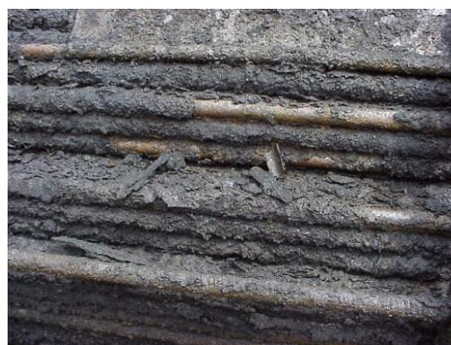
Fig. 1 Photo of shell-side fouling of refinery heat exchanger (Coletti et al. 2015). Reproduced with permission (Copyright 2015 Elsevier).
