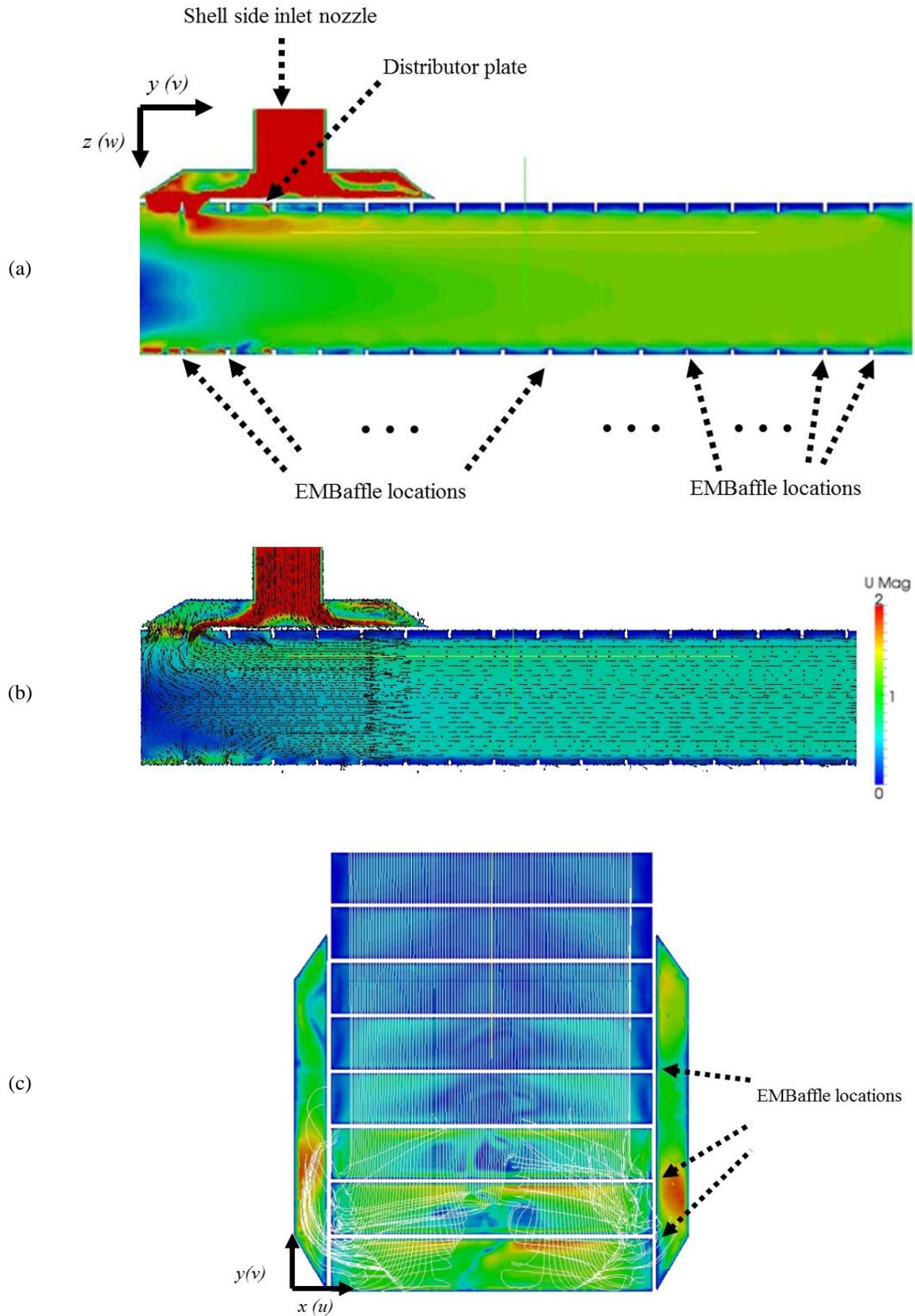
Fig. 2 Velocity field in the tube bundle coloured according to the velocity magnitude. (a) longitudinal cross section of EMBaffle with velocity field, (b) direction of velocity vector, and (c) flow field through cross section of the EMBaffle bundle immediately below the flow distributor.
