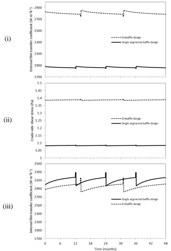
Fig. 11 Profiles of (i) external transfer coefficient, (ii) equivalent crude-side shear and (iii) internal transfer coefficient. Solid and dashed lines represent segmental baffle and EMbaffle heat exchangers, respectively
