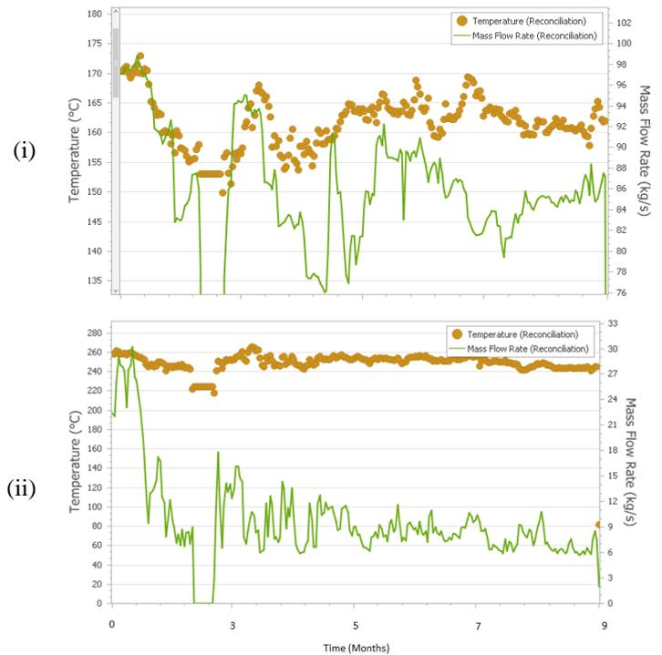
Fig. 6 Reconciled data for segmental baffle exchanger. Inlet temperature and mass flow rate profiles of (i) crude stream and (ii) LCR stream.
