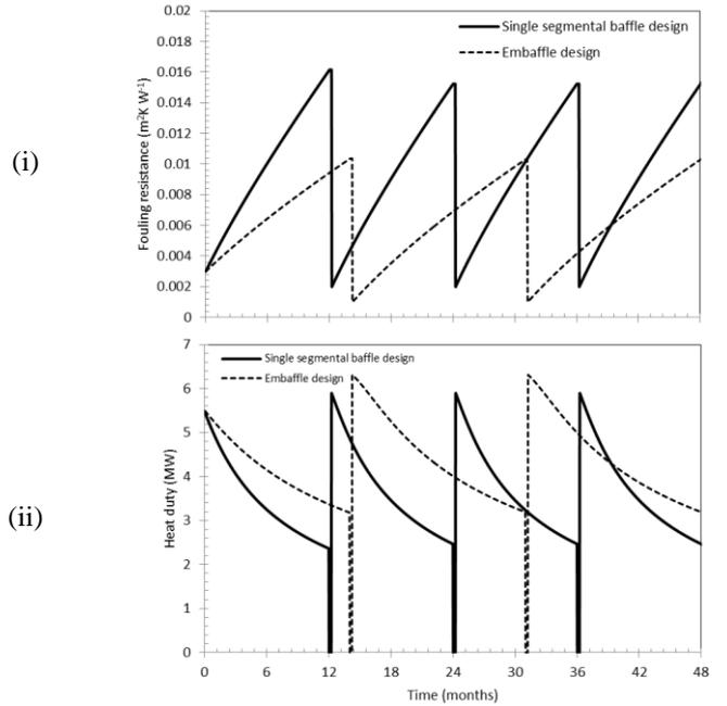
Fig. 10 Comparison of performance for Segmental baffle and EMbaffle units: (i)  $R_f$  and (ii) heat duty.
