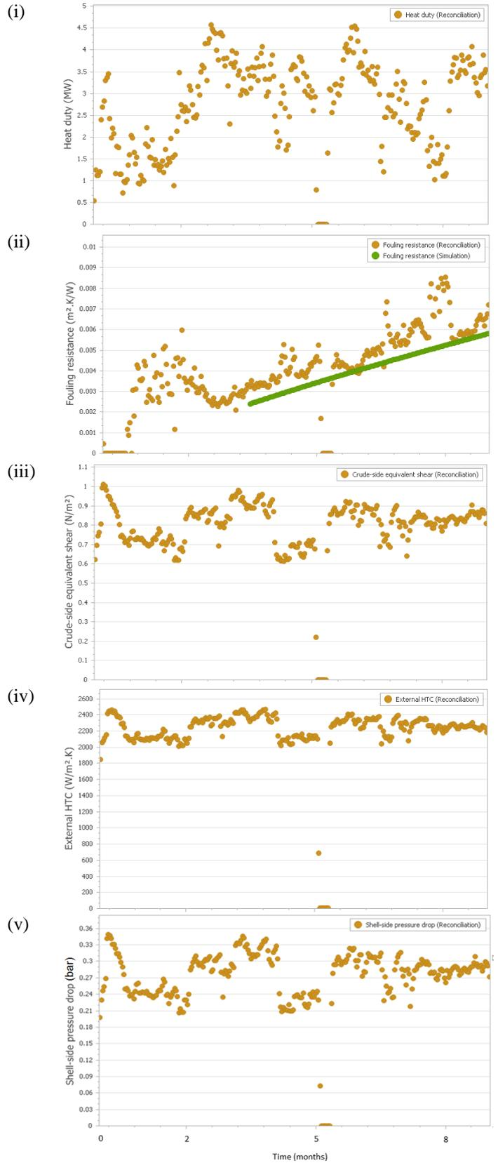
Fig. 9 Operational profiles for EMbaffle unit: (i) heat duty, (ii)  $R_f$ , (iii) shear stress, (iv) external transfer coefficient, and (v) shell-side pressure drop.
