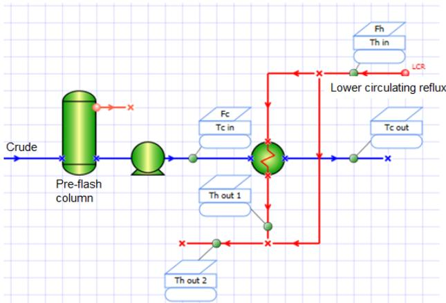
Fig. 5 Illustration of heat exchanger instrumentation.  $F_c$  and  $F_h$  are cold and hot stream flow measurements, respectively.  $T_c$  and  $T_h$  are cold and hot stream temperature measurements, respectively. 'in' and 'out' denote inlet and outlet streams.
