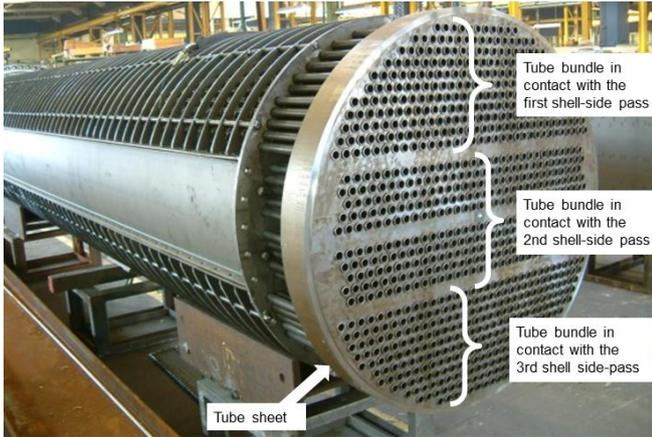
Fig. 3 EMbaffle three-shell-pass bundle.
