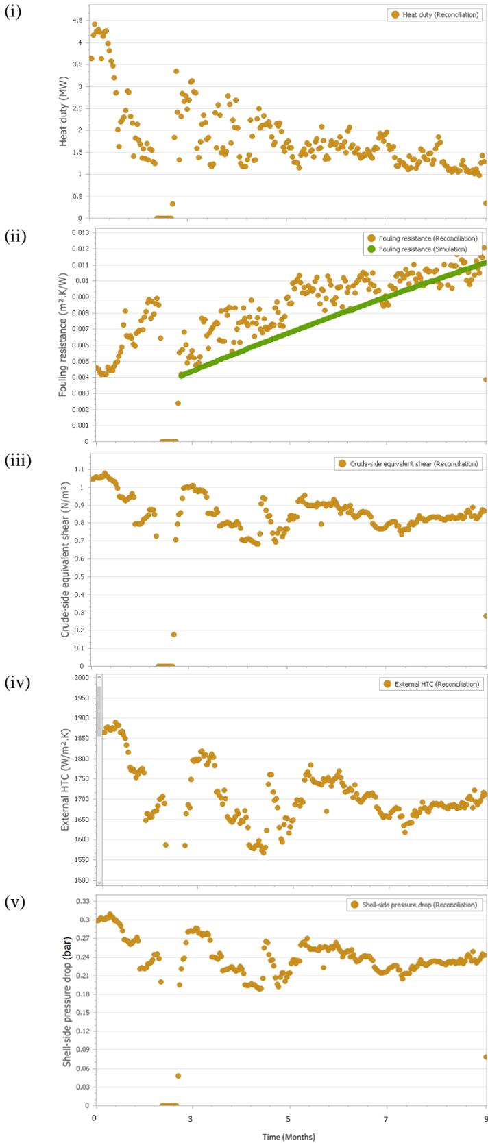
Fig. 8 Operational profiles for single segmental baffle unit: (i) heat duty, (ii)  $R_f$ , (iii) shear stress, (iv) external transfer coefficient, and (v) shell-side pressure drop.
