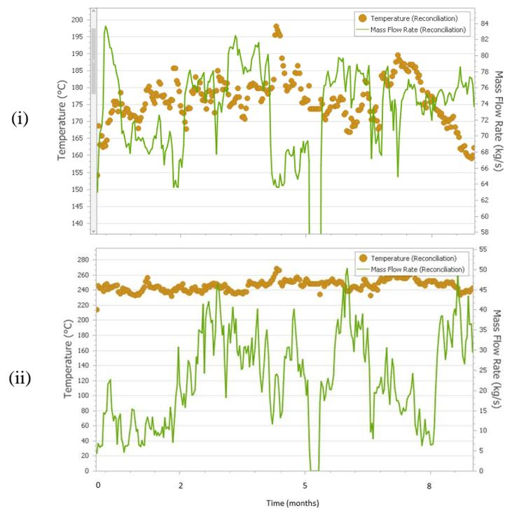
Fig. 7 Reconciled data for EMBaffle exchanger. Inlet temperature and mass flow rate profiles of (i) crude stream and (ii) LCR stream.
