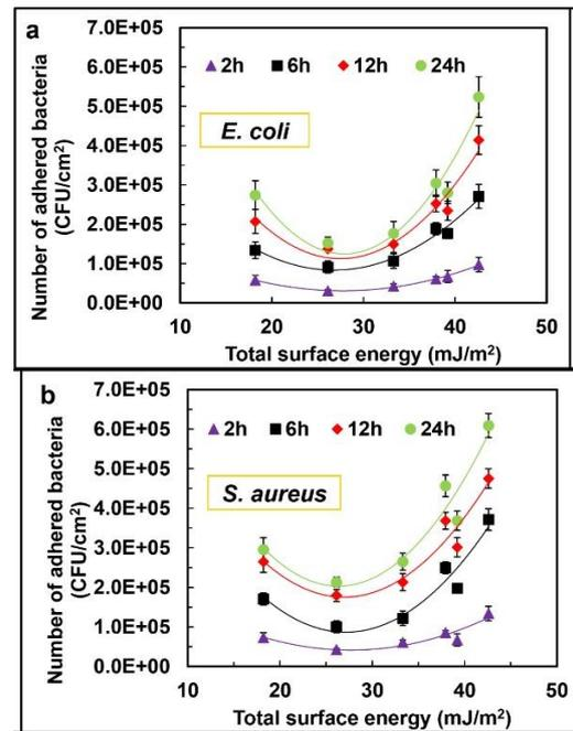
Figure 3. Effect of surface energy on (a) *E. coli* and (b) *S. aureus* adhesion at various contact times (N = 10, bars are standard error of the mean).
