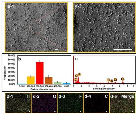
Figure 2. (a) SEM images of TiO<sub>2</sub>-PTFE nanocomposite coatings at two different magnifications (scale bars correspond to 5  $\mu$ m); (b) Size distribution of the PTFE particles; (c) Semi-quantitative results of EDX; (d) EDX mappings of the a-1 SEM image (scale bar corresponds to 5  $\mu$ m). Typical images are shown from one of several examinations.
