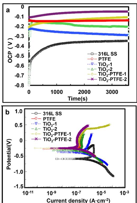
Figure 4. (a) Open-circuit potential characteristics and (b) potentiodynamic polarization curves of different samples in NaCl solution.
