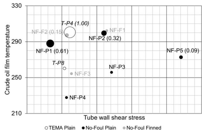
Fig. 4 Fouling experiment results for plain and helically finned tubes.
