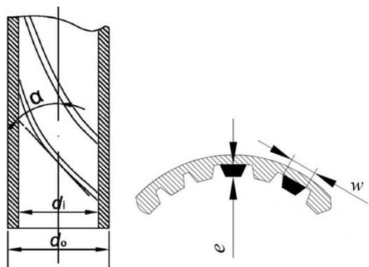
Fig. 1 Geometry description of a helically-finned tube (Ji et al., 2012).
