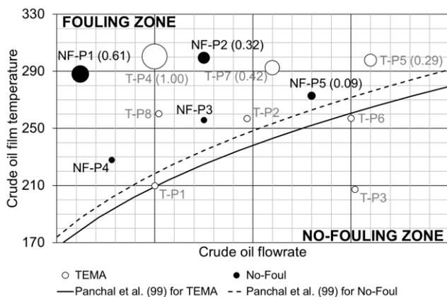
Fig. 3 Fouling experiment results for TEMA and *No-Foul* heat exchangers as a function of crude oil flowrate.
