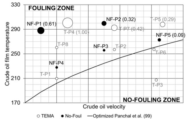
Fig. 2 Fouling experiment results for the TEMA and *No-Foul* heat exchangers as a function of crude oil velocity.
