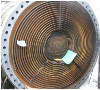
Fig. 2 - An opened spiral produced water cooler at Statoil's Leismer SAGD facility near Fort McMurray AB.
