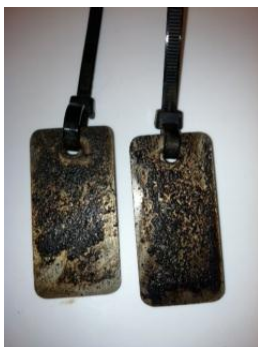
Fig. 8 – Image of fouled coupons following a boil-off test of SAGD BFW. Coupons were laid horizontally on the bottom of the beaker.
