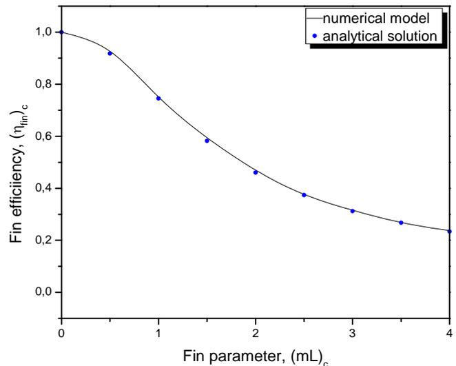
Fig. 6 Comparison between numerical and analytical solutions for fin efficiency for clean convective heat transfer.
