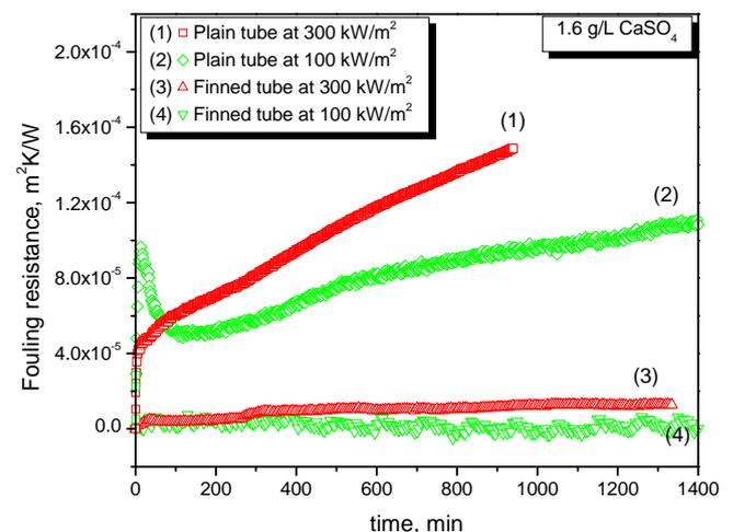
**Fig. 1** Comparison of fouling resistances for plain stainless steel and annular finned Cu-Ni tubes at 100 and 300 kW/m<sup>2</sup> for a CaSO<sub>4</sub> concentration of 1.6 g/L (Esawy, 2011).
