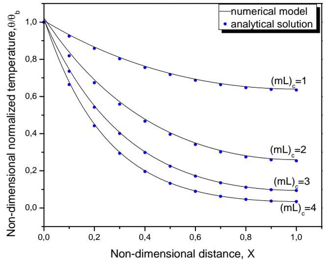
Fig. 5 Comparison between numerical and analytical solutions for fin temperature distribution for clean convective heat transfer.
