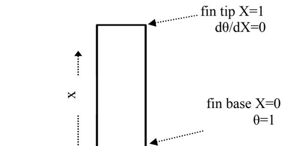
Fig. 4 Boundary conditions for the simulated fin.
