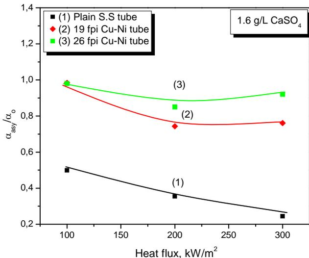
**Fig. 2** Relative drop of heat transfer coefficient versus heat flux at time of 1350 min for 19 and 26 fpi annular finned tubes and a smooth tube, for a  $\text{CaSO}_4$  concentration of 1.6 g/L (Esawy et al, 2010).
