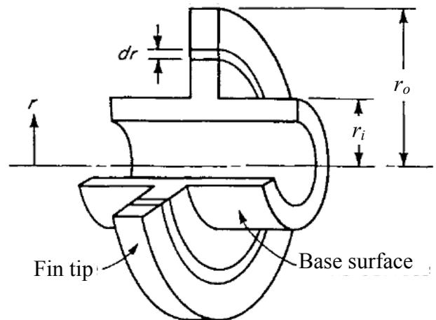
**Fig. 3** Geometry of the simulated annular fin.
