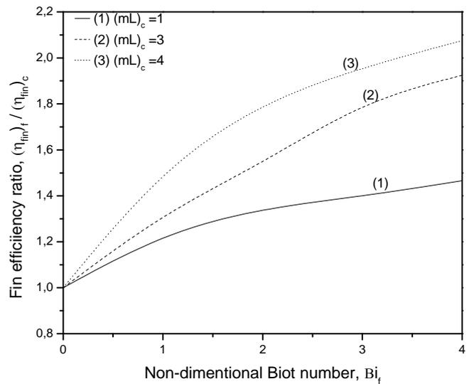
**Fig. 9** Fouled to clean fin efficiency ratio versus non-dimensional time for different clean fin parameters during nucleate pool boiling.
