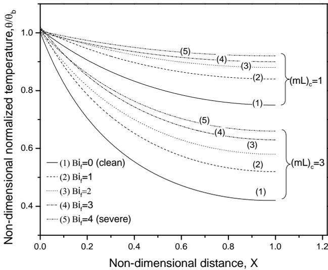
**Fig. 7** Effect of fouling on fin temperature distribution during nucleate pool boiling.
