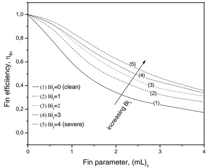
**Fig. 8** Effect of fouling on fin efficiency during nucleate pool boiling.
