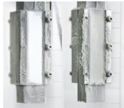
Figure 6 Scaling test in saturated CaSO 4 solution after 24 h Left: CVD-coated shiny aluminum plate without deposits Right: crystal growth on the entire surface of the uncoated reference piece
