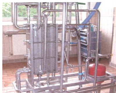
Fig. 2 Pilot plant used for practical tests (Institute of Food Quality LUFA-Oldenburg) with GEA Ecoflex VT04 plate heat exchanger.
