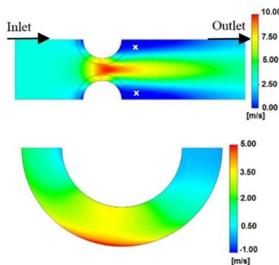
Fig. 5. Axial velocity distribution with 3 m/s inlet air velocity (top) and in the metal foam (below)
