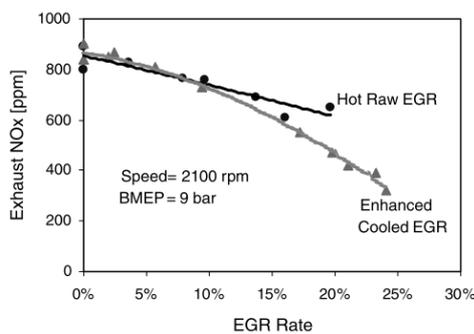
Fig. 2. Exhaust NO<sub>x</sub> emission vs. EGR rate (Zheng et al., 2004)
