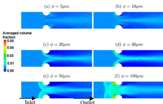
Fig. 6. Average volume fraction of particle with particle size distribution
