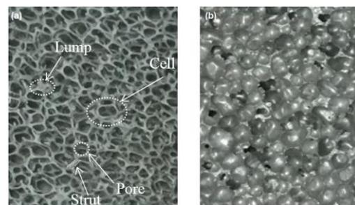
Fig 1. (a) 10 PPI open-cell metal foam (b) Closed-cell metal foam
