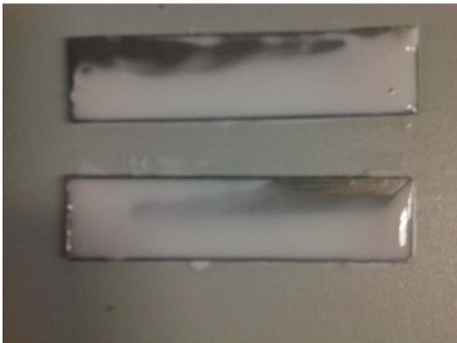
Fig. 19: Fouling layer on a cooled surface of stainless steel caused by 55 wt-% polymer dispersion.
