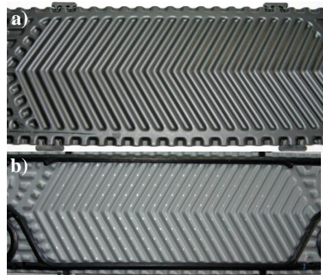
Fig. 6 Appearance of two coated M3 plates after the wear test: a) rating 0; b) rating 3
