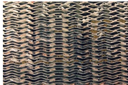
Fig. 18 Appearance of the channels on the tap water outlet side.
