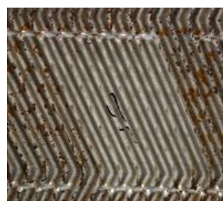
Fig. 11 Area of a coated plate cleaned with a dry cloth showing that the easy to clean and repellent properties of the coating remained intact after 5 months in operation.
