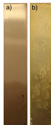
Fig. 2 Appearance of two coated coupons after being immersed in water at high temperature for 2 weeks: a) no blisters; b) large blisters on the entire surface.
