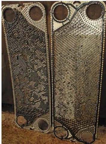
Fig. 12 Amount of fouling on the: a) uncoated and b) coated plates.
