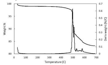
Fig. 1 TGA curve of HTSG coating measured in air.
