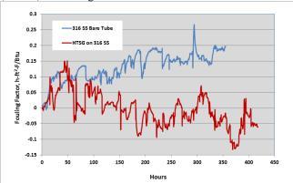
Fig. 4 Comparison of fouling rate for bare SS316 tube (blue) and tube coated with HTSG (red) at 600  $^{\circ}$ F in flowing crude oil
