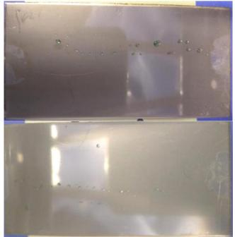
Fig. 3 Samples of HTSG coating after 6 h steam exposure Drops on the sample are from the test ink.
