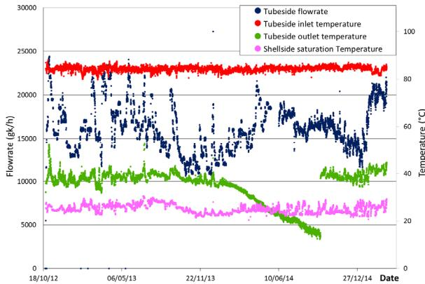
**Figure 5:** Raw data recorded over the 2 years operation, calculated with Edgeview – quench water inlet & outlet temperatures, quench water flowrate and C3 saturation temperature
