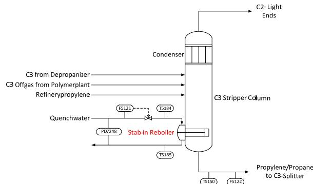
**Figure 1:** C3 Stripping unit with stab-in HEX and instrumentation
