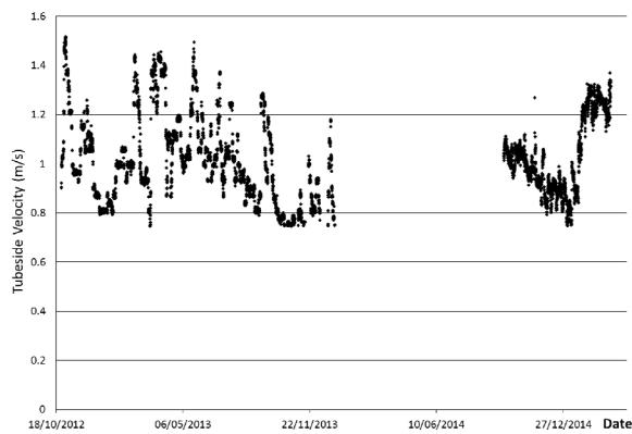
**Figure 7:** Quench water tubeside velocity over the 2 years operation, calculated with Edgeview based on filtered data
