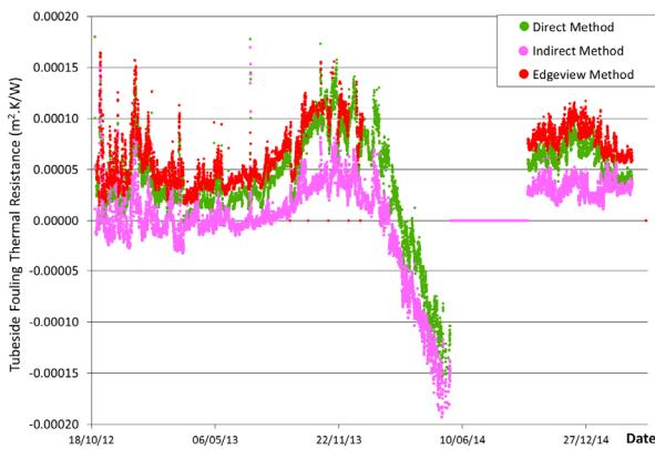
**Figure 2:** Tubeside fouling thermal resistance. Direct, Indirect and *Edgeview* Methods
