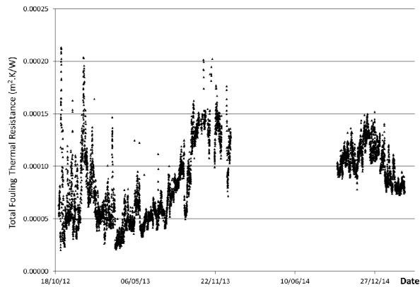
**Figure 4:** Global fouling thermal resistance calculated with *Edgeview* over the 2 years operation
