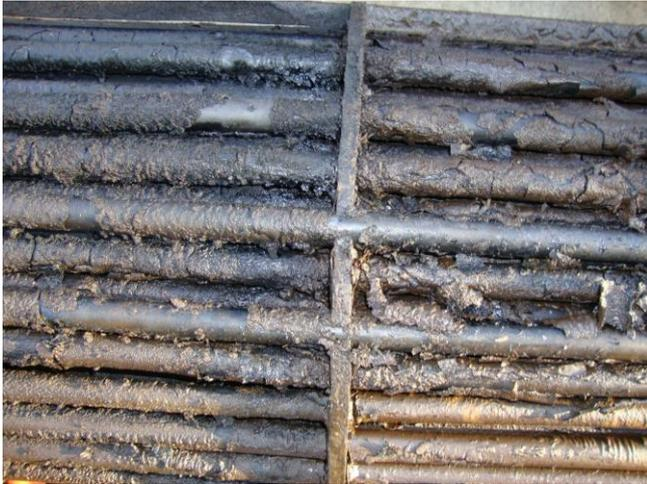
Fig. 2 Tube bundle extracted removed from hot exchanger, heavy fouling (feed on the shell side).
