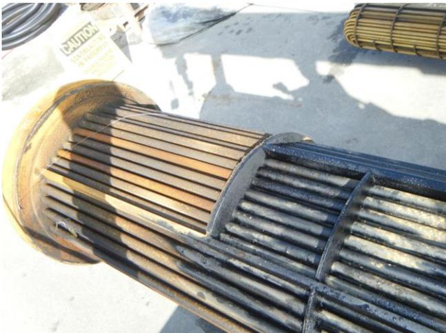
Fig. 4 Tube bundle removed from cold exchanger, nearly no fouling (feed on the shell side)
