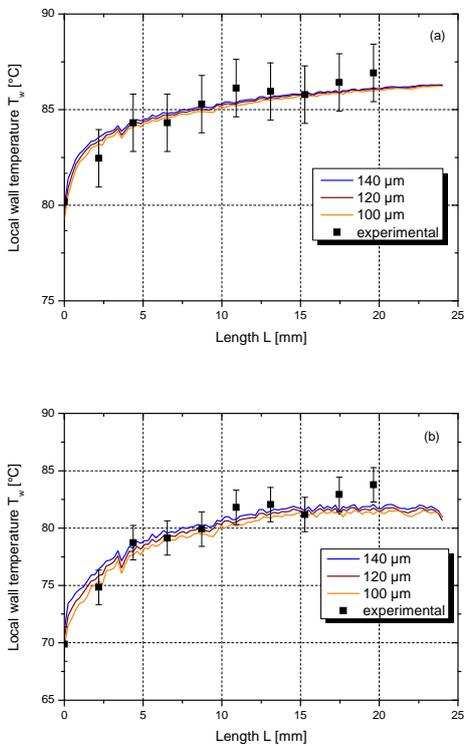
Fig. 10 Experimental vs. simulation results of the local temperature measurements: (a)  $2.1 \cdot 10^{-5} \text{ kg s}^{-1}$ , (b)  $1.4 \cdot 10^{-4} \text{ kg s}^{-1}$ .
