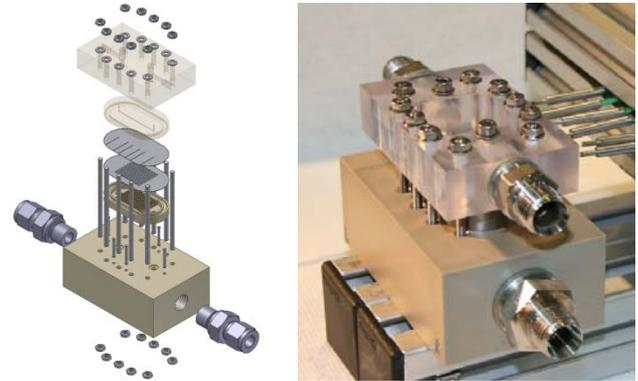
**Fig. 4** Schematic exploded draft of the experimental micro heat exchanger (left) and assembled experimental micro heat exchanger for fouling investigation (right).
