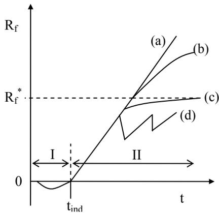
**Fig. 2.** Fouling resistance over time: I induction period, II layer growth period; (a) no removal, (b) decreasing deposition rate due to removal, (c) asymptotic behavior: deposition and removal rate become equal, (d) saw tooth shape: removal of bigger deposit fractions.
