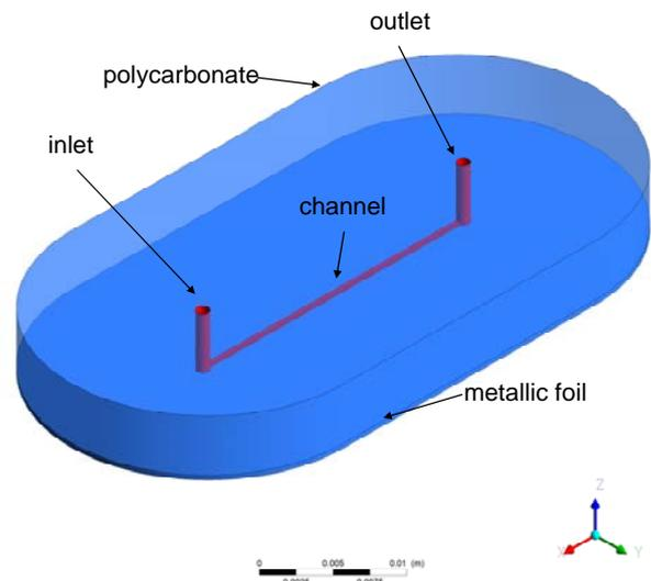
Fig. 8. Geometric model of the flow system: micro channel in polycarbonate with metallic bottom side.
