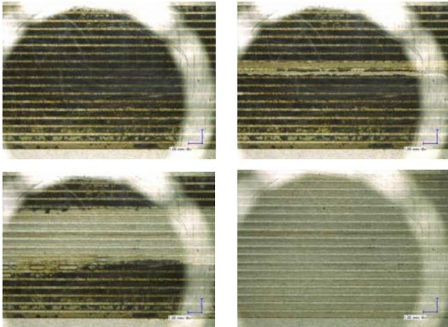
Fig. 14 CIP (HCl 6 wt-%) of a 18 micro structure channels fouled with CaCO<sub>3</sub>; from top left to bottom right (0 min; 10.5 min; 16.5 min; 18.5 min) 20x magnified, flow from right to left.
