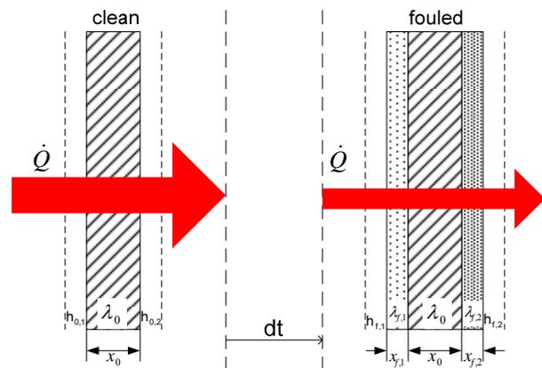
Fig. 1 Schematic diagram of the heat flux through a clean and a fouled heat exchanger wall.
