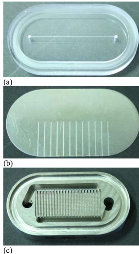
**Fig. 5** Micro structured devices: (a) polycarbonate element with one micro channel, (b) heat transfer foil with 12 micro slots for thermocouples, (c) titan element for heating with 693 channels.
