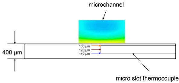
Fig. 9 Schematic profile for the micro channel and the metal foil with a micro slot. Arrows mark the possible measuring points of the thermocouple in the micro slots of the heat exchanger foil.
