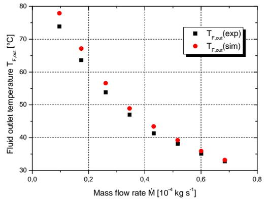
Fig. 11 Fluid temperature at the outlet versus the mass flow rate.
