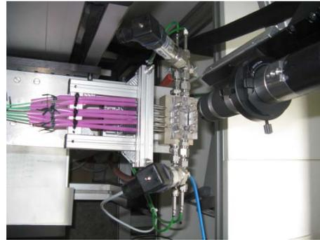
Fig. 7 Setup of micro heat exchanger with digital microscope at right (view from top).
