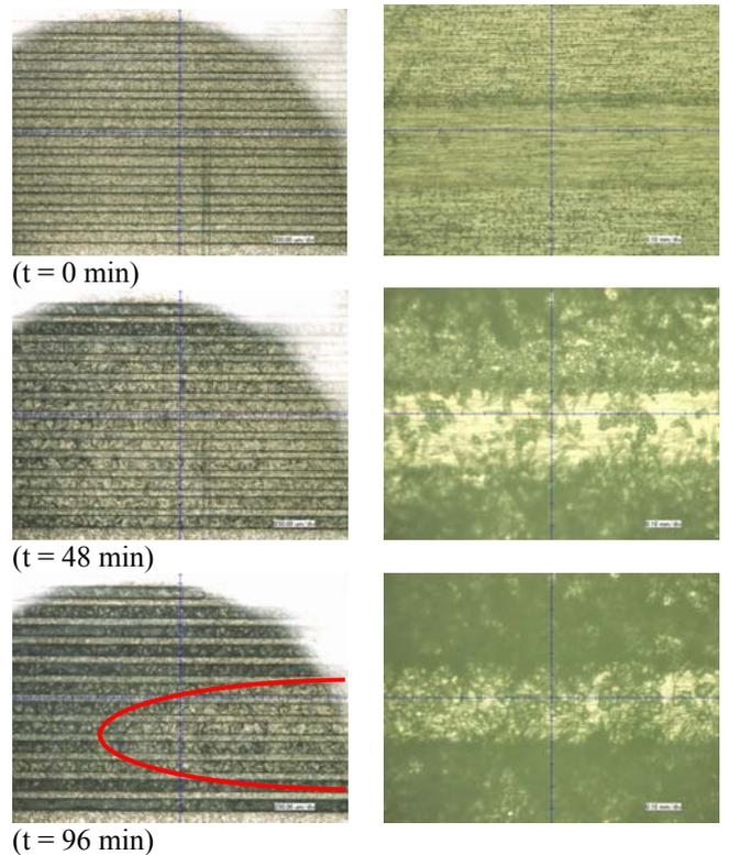
Fig. 12  $\text{CaCO}_3$  in micro structures over time (flow from right to left, crystals appear dark). Left column: 12 channels ( $40 \text{ ml min}^{-1}$ ,  $T_m = 60 \text{ }^\circ\text{C}$ ; 30x magnified, parabolic fouling
