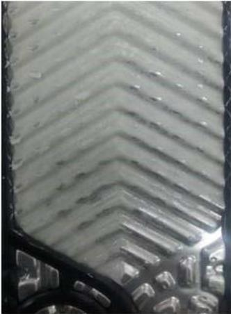
Fig.9 Visualization of  $CaSO_4$  crystallization fouling on the heat transfer surface.
