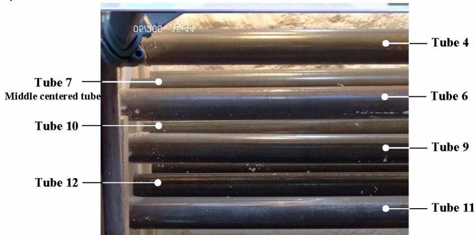
Fig. 3. The staggered arrangement of the heat exchanger tubes. Tube 7 is the middle centered tube of the heat exchanger.
