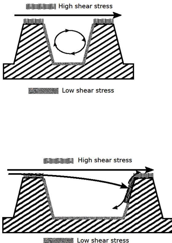
Fig. 8 Flow patterns over different internal structure geometries.
