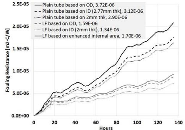
Fig. 6 Measured fouling resistance based on different surface areas for the plain and LF tubes. Fouling rates (the slope of each line) are shown in the legend in the units of [m<sup>2</sup>-C/W/day].
