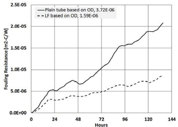
Fig. 4 Post induction fouling resistance trend for enhanced and plain tube. Fouling rates in units of  $\text{m}^2\text{-C/W/day}$  are shown in the legend.
