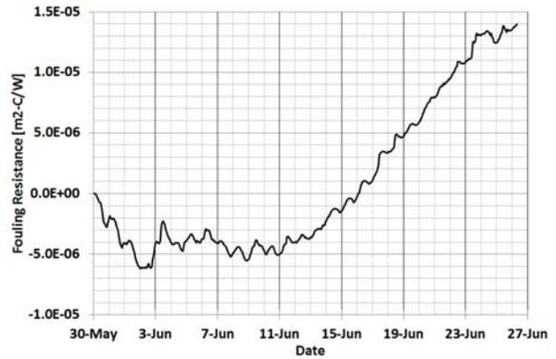
Fig. 3 Steady state fouling resistance trend for the LF enhanced tube.
