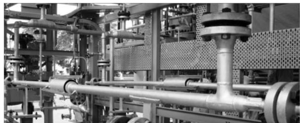
Fig. 2 Photo of Fouling Test Section.
