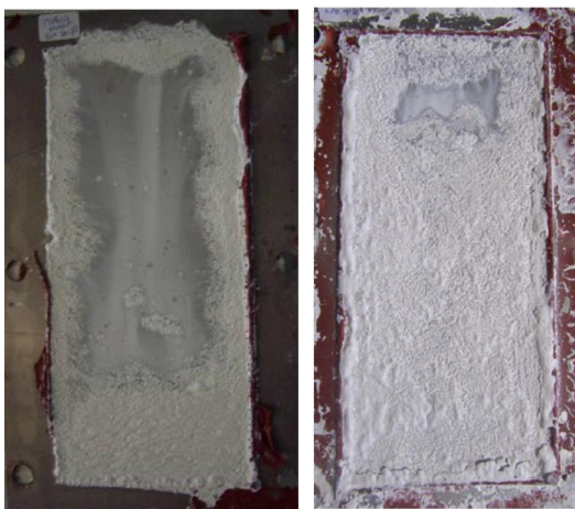
Fig. 10. Experimental results for deposition profiles. On the left: T_{\text{fluid}}=353 \text{ K} , 0.8 lps, 20 \text{ kW}/\text{m}^2 , s.c. 50.7%. On the right: T_{\text{fluid}}=333 \text{ K} , 0.45 lps, 30.2 \text{ kW}/\text{m}^2 , s.c. 50.7%. Flow is directed downwards.
