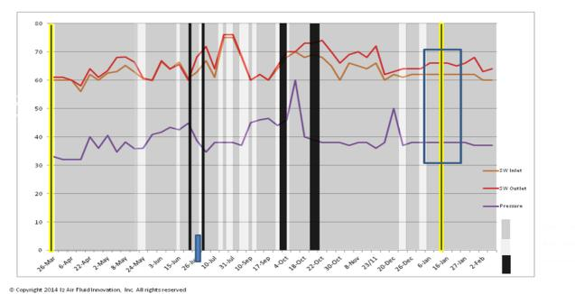
Figure 2: Pressure and temperature chart LPAC # 1
