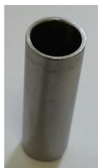
Fig. 1. Picture of the tube-sample used for \beta -Lg thermal denaturation experiments
