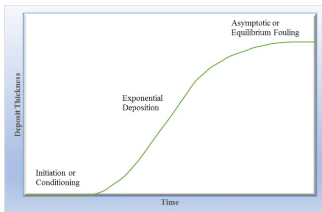
Fig. 1 Idealized change of fouling layer thickness in time (Bott, 2001)
