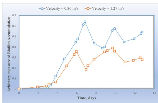
Fig. 2 The effect of flow velocity upon the actual thickness of fouling layer in time (Bott, 2001)
