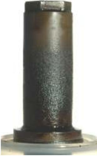
Fig. 2 The heated test probe partially covered with deposit
