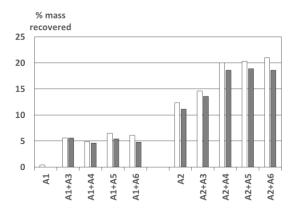
Figure 2a: Ratio of the mass of blocked particles recovered (floor, outer surface and sub-surface) (white) and fouling particles (outer surface and sub-surface) (grey) to the total mass of particles introduced into the air stream for different binary mixtures (exchanger A).
