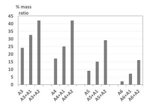
Figure 5: Ratio of the mass of larger particles in the sub-surface region to the total mass of particles introduced for different mixtures. (Exchanger A).
