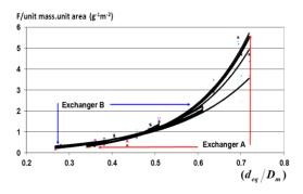
Figure 7: Variation of the fouling factor per unit mass and unit exchanger surface area as a function of non-dimensional equivalent particle size for all binary mixtures of particles examined in both exchangers. (Air speed is 5m/s).
