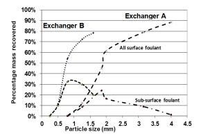
Figure 6: Evolution of the mass of foulant recovered on the exchanger surface as a function of particle size for discrete size ranges. Taken from Haghighi-Khoshkhoo & McCluskey 2007 with kind permission.
