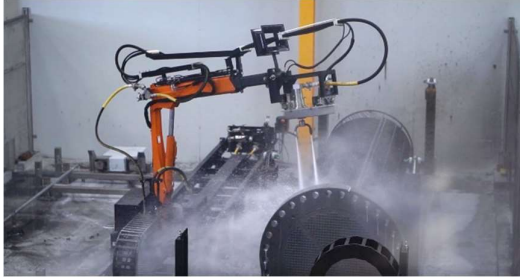
Figure 2. Automated and remotely operated shell-side rinsing of a heat exchanger as viewed from the control room
