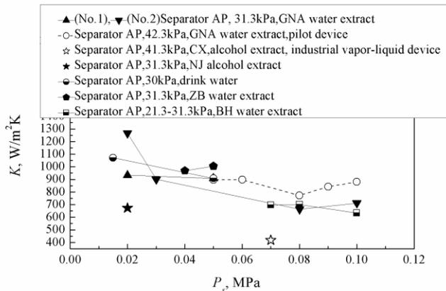
Fig.2 Overall heat-transfer coefficient  $K$  of the industrial scale fluidized bed evaporator and gauge pressure of the boiler steam for different concentration liquids of traditional Chinese medicines.
