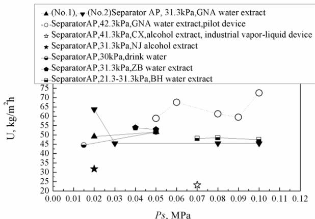
Fig.3 Evaporation intensity  $U$  of the industrial scale fluidized bed evaporator and gauge pressure of the boiler steam for different concentration liquids of traditional Chinese medicines.
