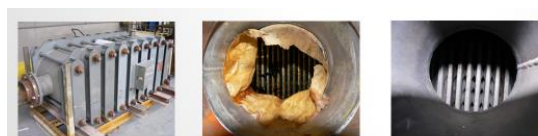
Fig. 9. Cleaning of a compabloc (e.g. polyacryl removal).
