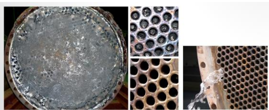
Fig. 7. Cleaning of a heat exchanger with fixed static mixers.
