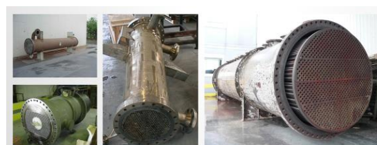
Fig. 6. Different types of bundles with fixed housing.
