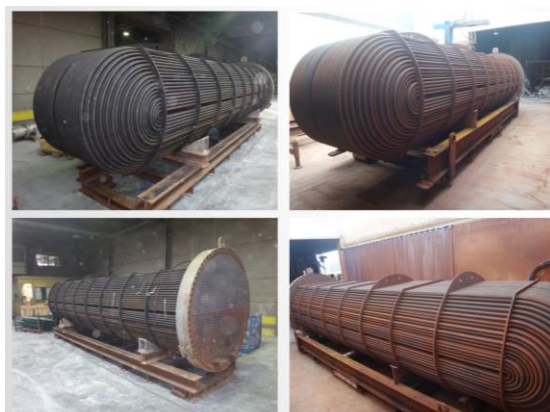
Fig. 15. Thermal cleaning after HP cleaning.
