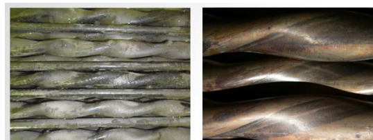
Fig. 10. Different types of bundles with twisted tubes iii .
