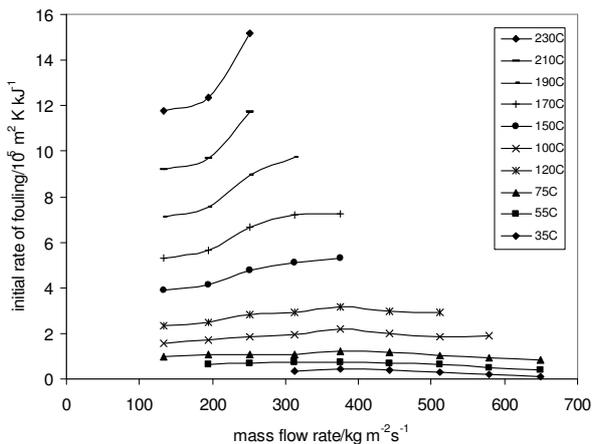
Figure 5 Initial fouling rates reported by Crittenden *et al.* (1987) for chemical reaction fouling of solutions of styrene in kerosene. The legend indicates initial surface temperature. Lines are solely to guide the eye.
