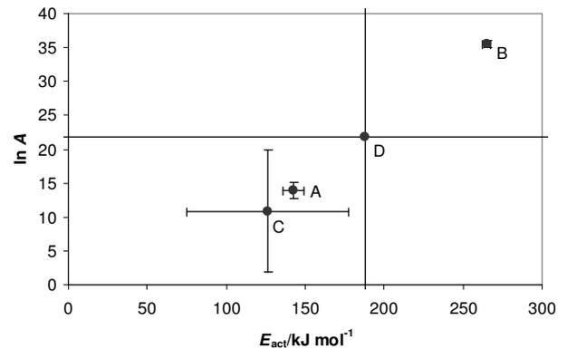
Figure 3 CE plot for the data in Figure 1. The error bars shown are the *standard errors* for the parameters obtained from linear regression. The error bars need to be far larger if 95% confidence intervals for the parameters are desired.
