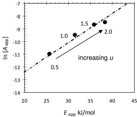
Figure 9 CE plot obtained for synthetic fouling rate data in Figure 8. Data labels show  $u$  values in  $\text{m s}^{-1}$ . The gradient of the dashed line is  $1/RT_{\text{ave}}$  and is plotted for comparison only.
