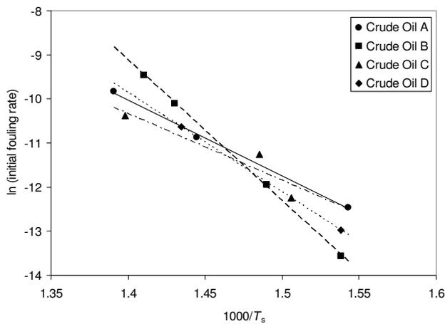
Figure 1 Pseudo-Arrhenius plot of data reported by Bennett *et al.* (2009) showing the initial fouling rates of four crude oils at different surface temperatures. There are four reliable data points for oil B, three for oils A and C, and only two for oil D. The lines were obtained by least squares regression to equation (1).
