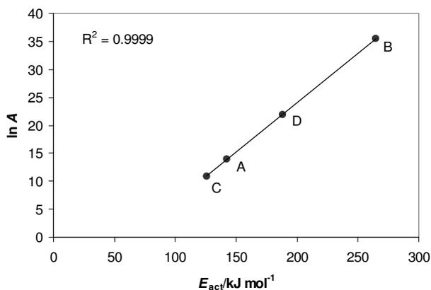
Figure 2 Compensation effect (CE) plot showing the Arrhenius parameters obtained from the data in Fig. 1. The straight line shows the linear regression fit to equation (2).
