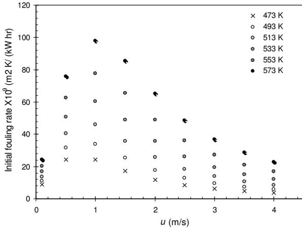
Figure 8 Synthetic fouling rate data generated using the Epstein fouling model for a model crude oil.
