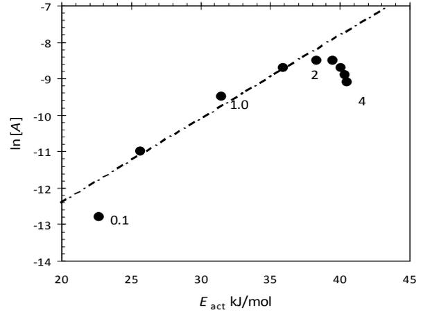
Figure 10. CE plot for all velocities in Figure 8. Data labels show selected  $u$  values in  $\text{m s}^{-1}$ . The gradient of the dashed line is  $1/RT_{\text{ave}}$ .
