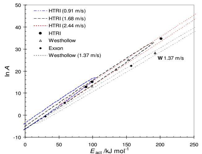
Figure 12 Selected CE plots for crude oil fouling tests reported by Panchal *et al.* (1997)
