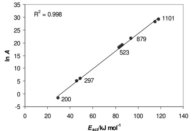
Figure 7 CE plot for fouling of lysozyme solutions using the data reported by Rose *et al.* (2000). Each data point derives from initial fouling rate measurements at a particular fluid velocity. Selected mass flow rates have been marked on the graph (in units of  $\text{kg m}^{-2} \text{ s}^{-1}$ ). The line is a straight line fit to the data points.
