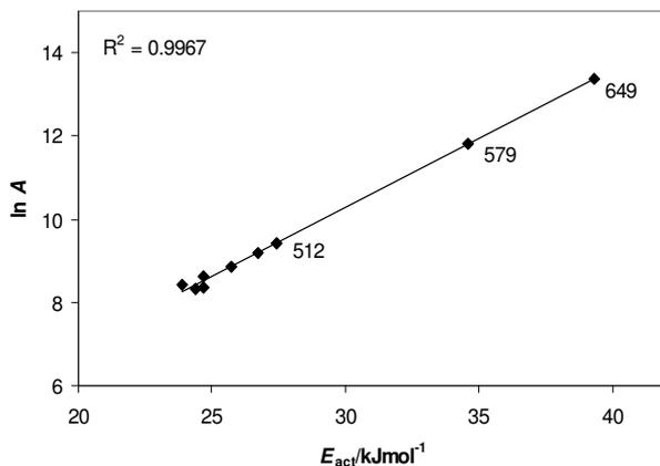
Figure 6 CE plot for styrene fouling data in Figure 5. Each data point derives from initial fouling rate measurements at a particular flow rate. Mass flow rates (in  $\text{kg m}^{-2} \text{ s}^{-1}$ ) are marked on selected data points. The line shows a straight line fit to the data.
