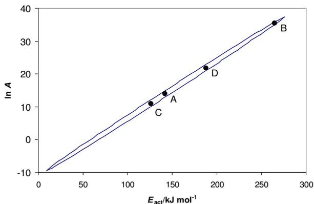
Figure 4 CE plot for the data in Figure 1 showing the 95% confidence ellipse for parameters of crude oil A. The gradient of the major axis of the ellipse is  $1/RT_{\text{ave}}$ , where  $T_{\text{ave}}$  is the harmonic mean of the temperatures employed in the kinetic study.
