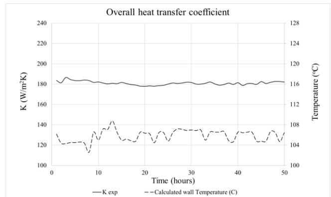
Figure 6. Experimentally determined heat transfer coefficient for hot pilot unit in the first test.
