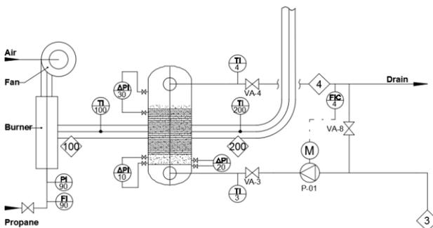
Figure 4. Schematic diagram hot pilot unit.
