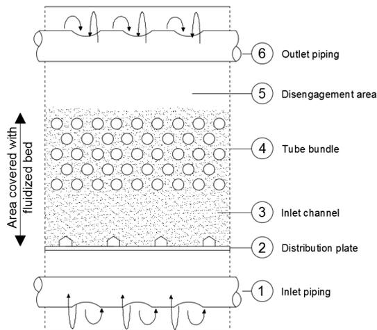
Figure 2. Schematic representation shell side fluidized bed heat exchanger with horizontal tubes.
