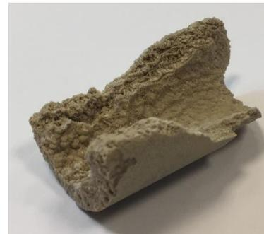
Figure 3. Sample of a fouling layer as found on the tube inlet of the brine heater of a Multi Stage Flash (MSF) Distiller at the Sabiyah plant.
