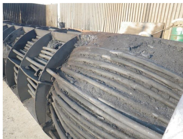
Fig.6. Exchanger damage due to popcorn polymer – bundle as extracted, with no cleaning
