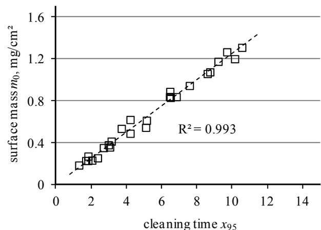
Fig. 3 Dependency of cleaning time and applied surface mass
