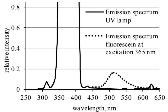
Fig. 2 Emission spectra of the UV lamp and the tracer
