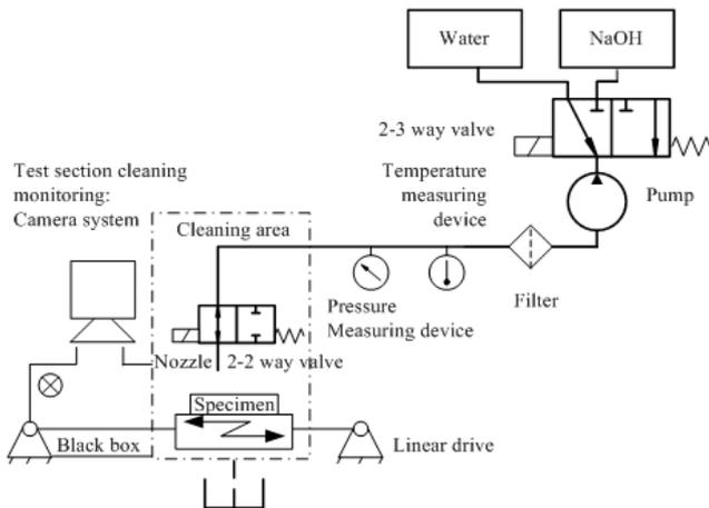
Fig. 1 Cleaning test rig with cleaning monitoring system
