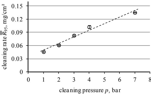
Fig. 5 Pressure dependency of the main cleaning rate by means of weighted mass
