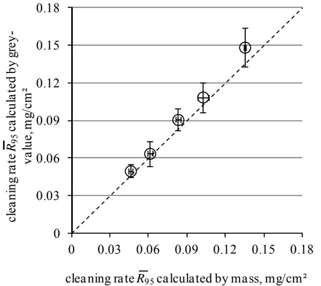
Fig. 6 Relationship between the main cleaning rates by means of weighted mass and grey-value
